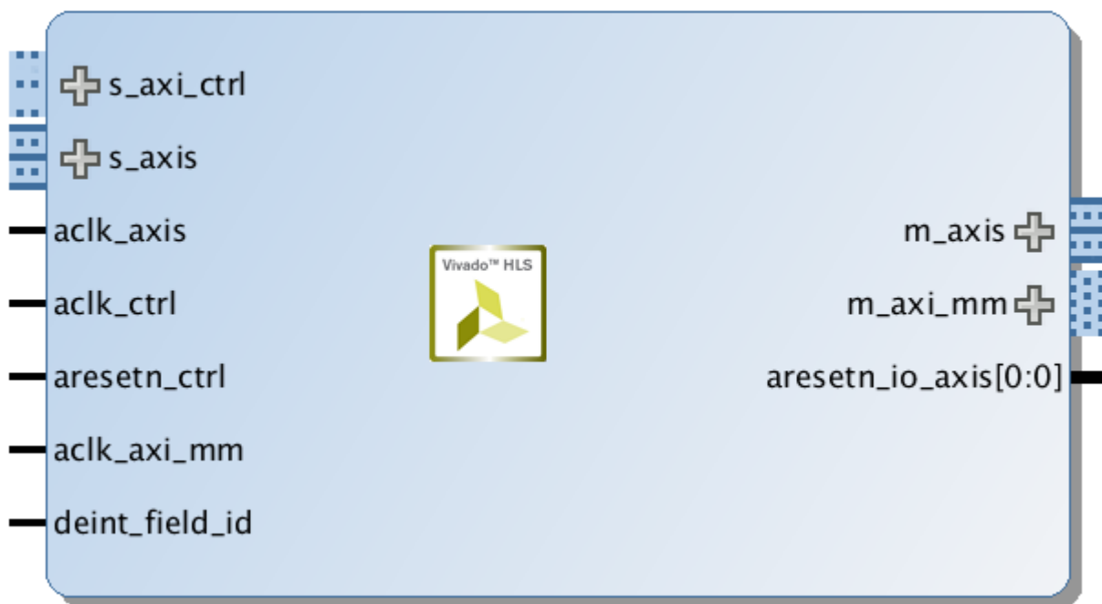
Figure 2-1: Full-fledged Video Processing Subsystem IP
