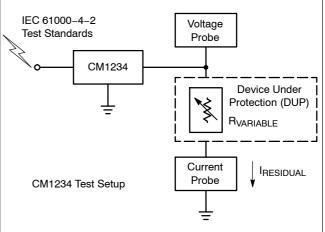
Figure 7. Test Setups: Standard Device (Left) and CM1234 (Right)
