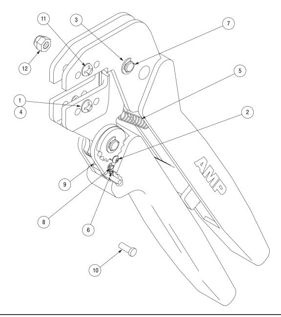
PRO-CRIMPER REPAIR KIT 679221-1● **QTY PER QTY PER** ITEM **DESCRIPTION** ITEM **DESCRIPTION ASSEMBLY ASSEMBLY** 1 SCREW, Die Retaining, M4 x 12 2 7 PIN, Pivot 3 2 SCREW, M3 x 4 1 8 PIN, Pawl 7 3 RING, Retaining 9 PAWL, Ratchet 1 4 SCREW, M4 x 14 10 PIN, Die Retaining 1 4 5 SPRING, Extension SCREW, Die Retaining, M4 x 25 1 11 1 6 SPRING, Extension 1 1 NUT, M4
