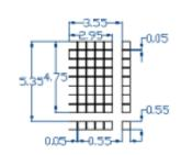
Figure 22: LCD Dimensional Drawing
