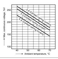
6.-(2) Ambient temperature vs Max. continuous voltage
