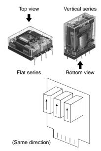
Cautions for close proximity mounting When using slim series in close proximity, mount all relays facing the same direction. Different mounting directions may cause change in the relay characteristics because NC relays are polarized.
