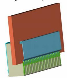
Figure 13 - Clip on cover shield
