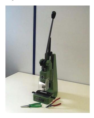
Figure 17 -- Connector Removal tooling HM2Y350
