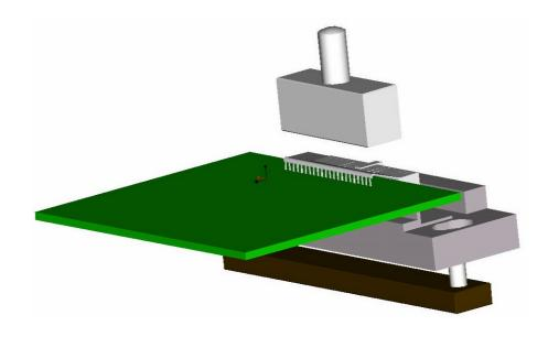
Figure 15 - One Piece Cover Shield Tool HM2Y509
