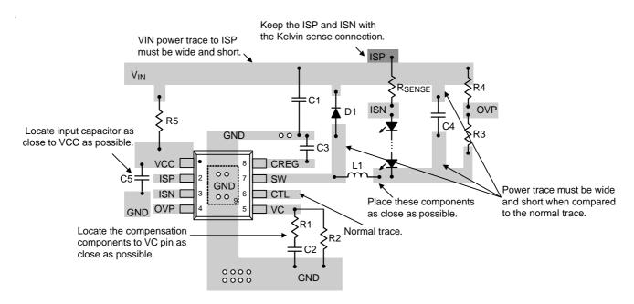
Figure 2. PCB Layout Guide
