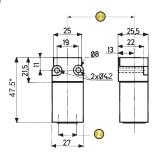
\* Allow 13 mm clearance to plug or to unplug when fixed
