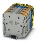
High-current terminal block, Blocked, Connection method: Push-in connection, Number of positions: 5, Cross section: 25 mm<sup>2</sup> - 95 mm<sup>2</sup>, AWG: 4 - 3/0, Width: 125 mm, Color: gray/blue/black-yellow, Mounting type: NS 35/15
