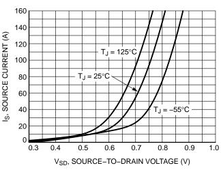
Figure 10. Diode Forward Voltage vs. Current
