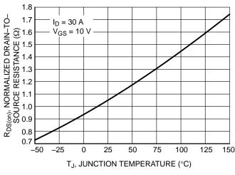
Figure 5. On–Resistance Variation with Temperature
