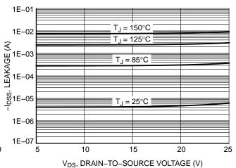
Figure 6. Drain-to-Source Leakage Current vs. Voltage
