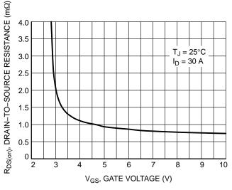
Figure 3. On-Resistance vs. Gate-to-Source Voltage
