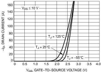
Figure 2. Transfer Characteristics
