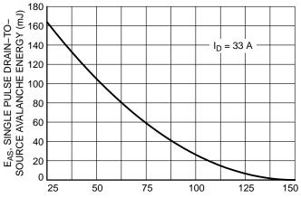
Figure 12. Maximum Avalanche Energy vs. Starting Junction Temperature
