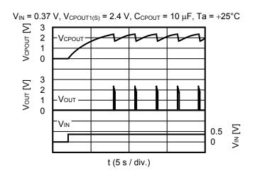
Figure 8 Startup Waveform for Intermittently LED Driving
