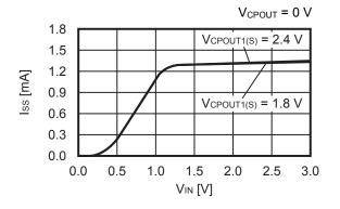
1.6 Current consumption during power-off (I<sub>SSS</sub>) vs. Input voltage (V<sub>IN</sub>)
