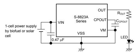
Figure 7 Intermittently LED Driving Circuit
