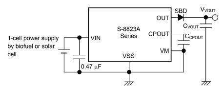
Figure 10 Circuit of Intermittently Power Supplying to Capacitor
