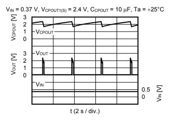
Figure 9 Steady-state Operation Waveform for Intermittently LED Driving
