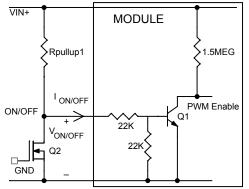
Circuit configuration for using negative On/Off logic
