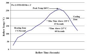
Recommended linear reflow profile using Sn/Ag/Cu solder.
