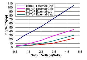
**Note:** Output ripple voltage for various output voltages with external 1x10 μF, 1x47 μF, 2x47 μF or 4x47 μF ceramic capacitors at the output (3A load). Input voltage is 12V.
