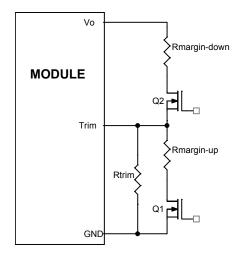
Circuit Configuration for margining Output voltage
