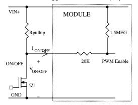
Circuit configuration for using positive On/Off logic
