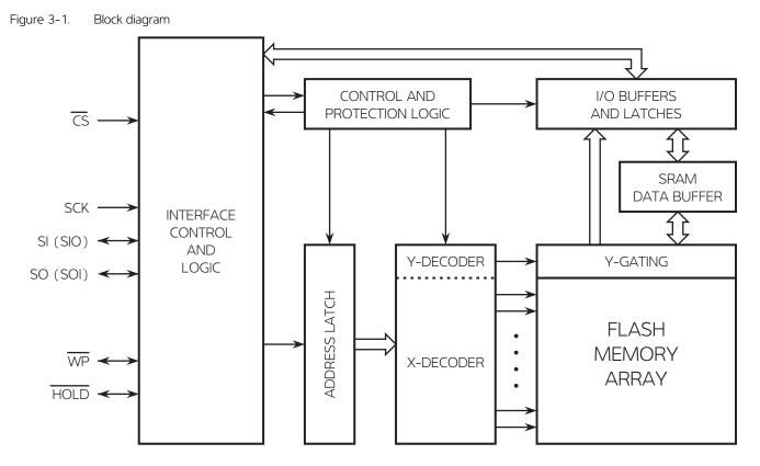
Note: SIO and SOI pin naming convention is used for Dual-I/O commands
